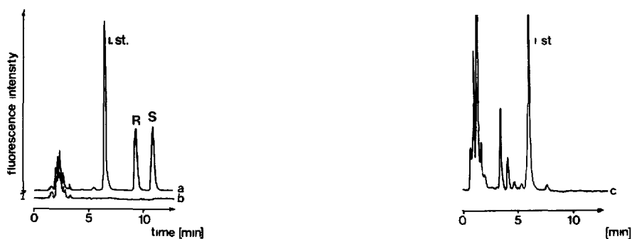
Fig. 2. Representative chromatograms for the separation of the diastereomeric carprofen derivatives in plasma samples 1 h after administration of 150 mg racemic drug. (a) Plasma concentrations: R -carprofen 2.9 \mu\text{g}/\text{ml} and S -carprofen 3.1 \mu\text{g}/\text{ml} . (b) Blank plasma sample. (c) Blank urine sample. i.st. = internal standard, naproxen.
